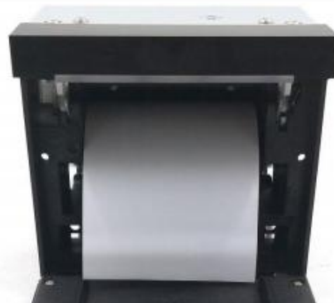
Fig. 4: Paper loading without roll spindle
