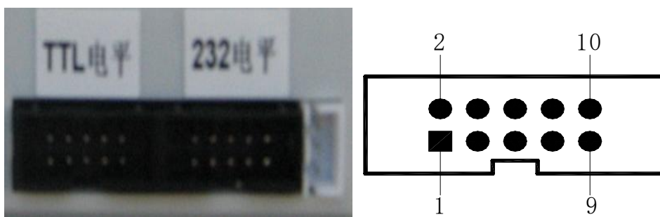
Figure 3-1 serial interface IDC10 pin type socket pin number 5PIN single serial interface socket of the serial number as shown in figure 3-2
